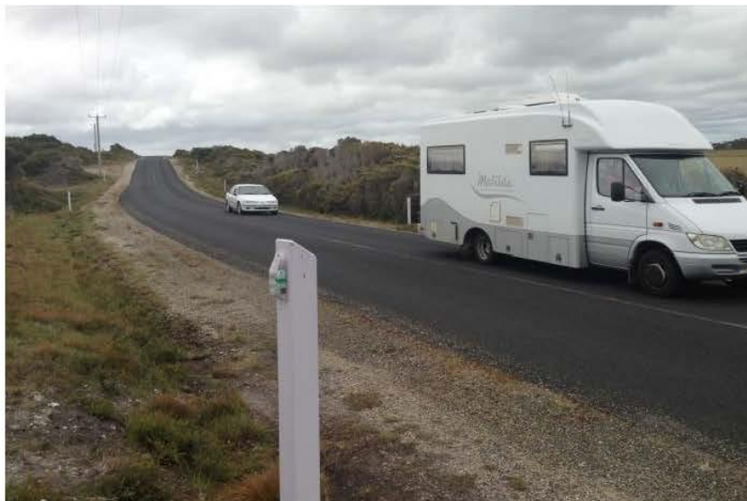
PHOTO: The alarm units that make up the virtual roadside fence are tripped by car headlights. (ABC News: Damian McIntyre)
