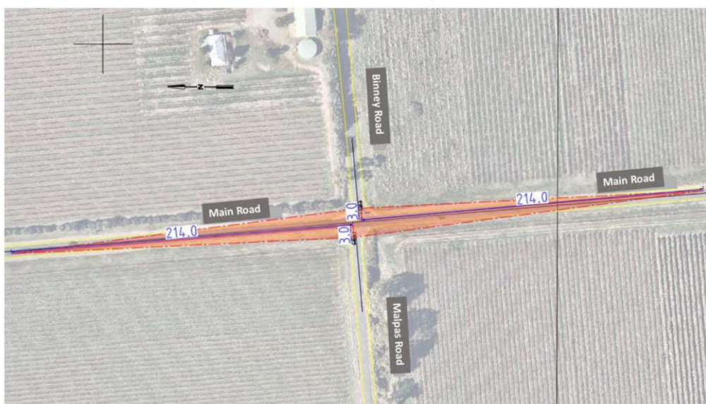
Figure 3.6: Main Road, Malpas Road & Binney Road SISD Diagram
