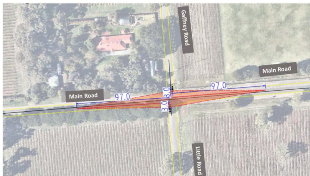
Figure 3.7: Main Road, Little Road & Gaffney Road SISD Diagram
