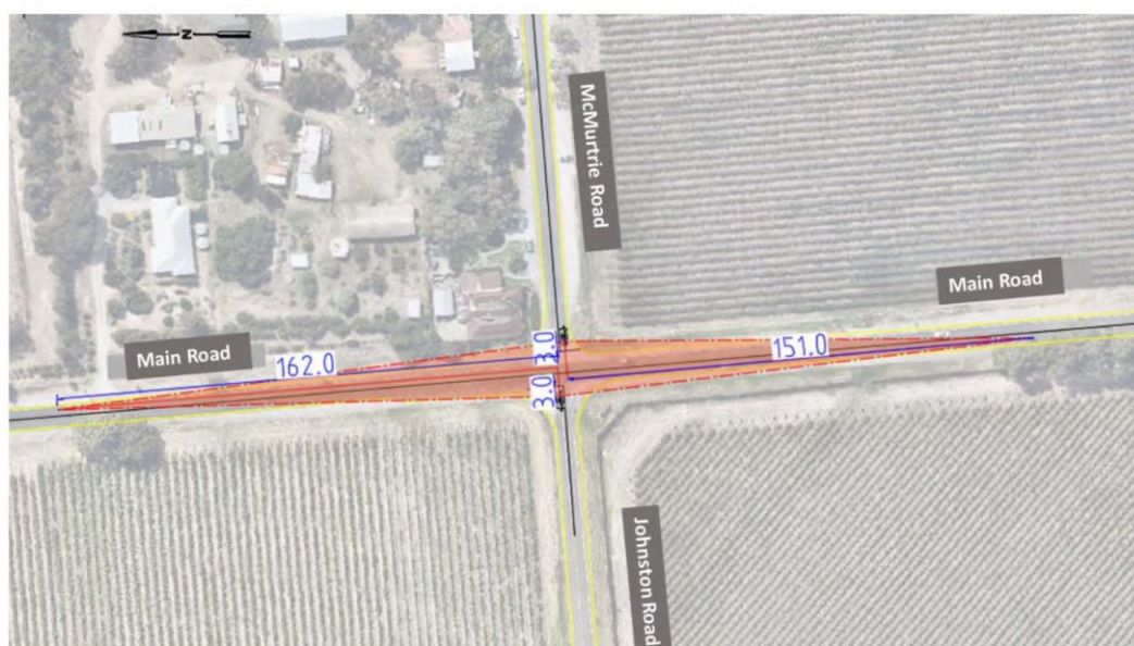
Figure 3.2: Main Road, McMurtrie Road & Johnston Road SISD Diagram
