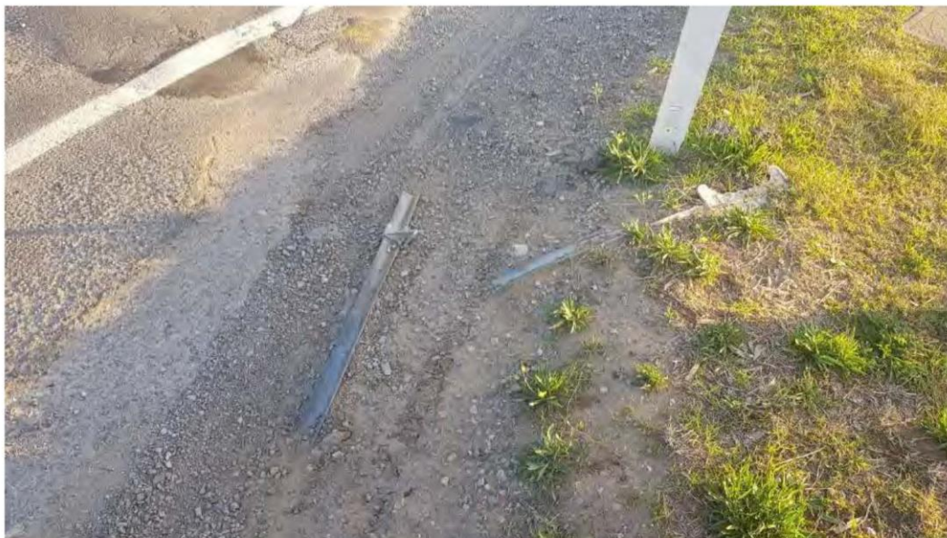
Figure 3.4: Fire Hydrant Marker Appears to Have Been Damaged by Rear Trailer Drag
